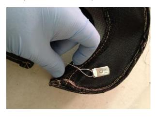
3. Install heat blanket around exhaust housing (shown off truck for display purposes) and snug it down by hooking safety wire around opposing loop to pull it tight. Please be aware, heat blankets on VGT turbos will require factory heat shield to be removed.
