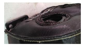
4. At this point, heat blanket is installed and functional. To keep it clean, we recommend using a damp rag and degreasing dish soap to clean grease/oil from the heat blanket. **DO NOT** use brake clean or any other flammable liquids to clean heat blanket, as it will act like a sponge and potentially cause a fire.
