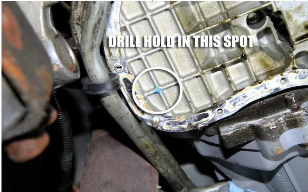
15. Drill a small pilot hole first for the large drill to follow. Then **drill with a 3/8" Bit.**
