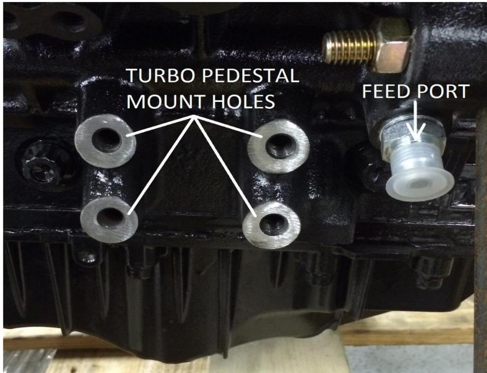
3. Next locate the 1/4" NPT X #4 JIC straight fitting. Apply Teflon Paste (**DO NOT use Teflon tape!**) to the threads and install into the turbo's center section feed port.
