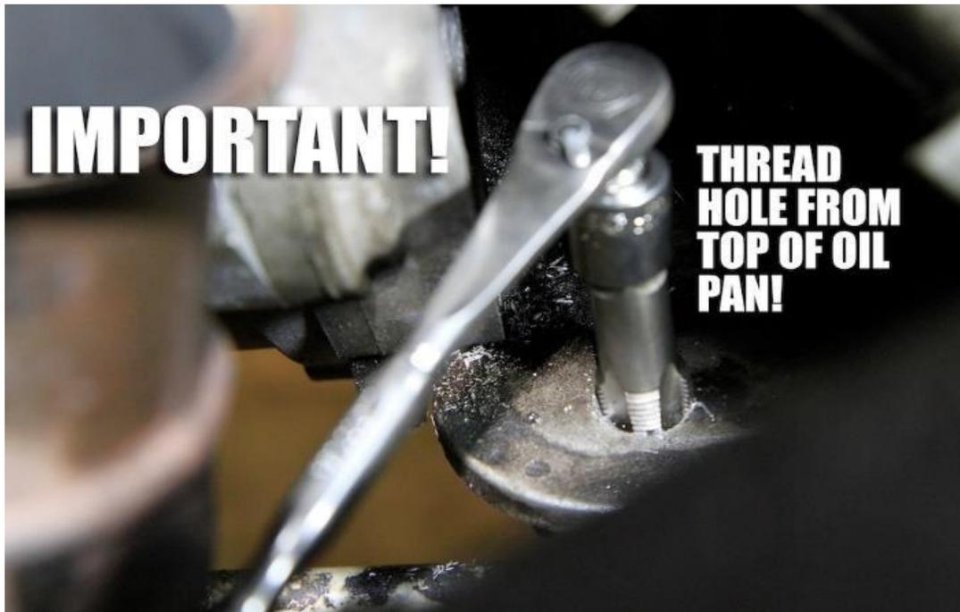
17. Thoroughly clean any debris from the drill and tapping process.
