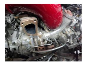
20. Place EGR cooler into position. **Do not start mounting bolts yet, just leave them in the** appropriate holes.
