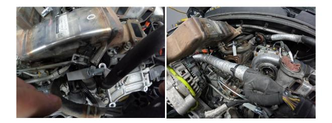
18. Install intake horn using supplied clamp. To ease install, use socket & extension to hold the clamp while turbo inlet is being placed into position.
