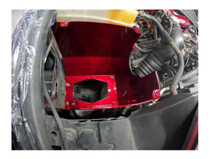
32. Install boot & clamp onto intake horn.
