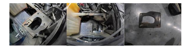
31. Install new air box using factory hardware.
