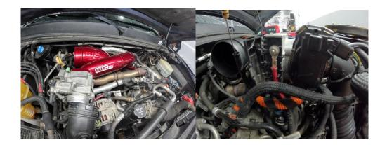
28. Due to size increase of intake horn, the temp sensor bracket for the connectors can be zip tied up to wire harness on firewall or to heater hose, but either way is fine.
