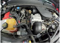
3. Remove the resonator from the turbo inlet by removing two 10mm bolts on resonator.
