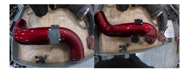
34. Place air filter in box & install pipe into boot first & air filter second before tightening clamps down. Once clamps are tight, plug in the MAF & CAC Temp Sensors.
