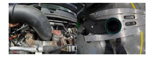
15. Disconnect EGR valve electrical connectors & four 13mm bolts to y-bridge to remove valve.
