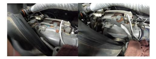
14. Loosen intake clamp & remove stock intake horn.
