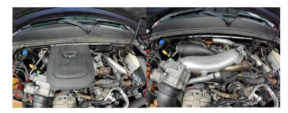
4. Remove the MAP sensor connector, intake air valve connector, grid heater connectors & battery cable from grid heater using a 10 mm socket.
