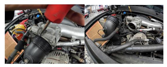
6. Loosen the four 10mm bolts on the intake air valve & remove from the truck.
