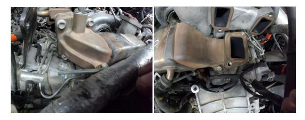
17. Remove hoses from front and rear section of front EGR cooler and remove from truck.
