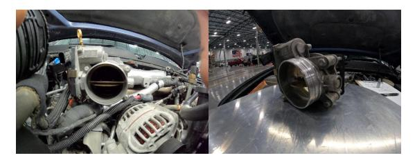
7. Remove two 13mm bolts from the bracket on the passenger side near engine oil dipstick. You may now remove the other two 13mm bolts from the flange at the engine side of the crossover pipe.
