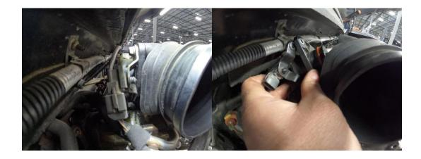
13. Loosen 13mm nut on turbo to allow solenoid wiring to move for access to horn clamp.
