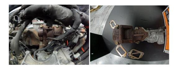
16. Remove mounting bolts for front EGR cooler as shown in picture (12mm & 13mm bolts).
