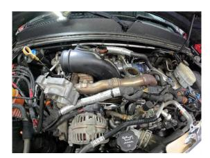
9. Remove grid heater from truck by removing the last 10mm bolt on the bottom left corner.
