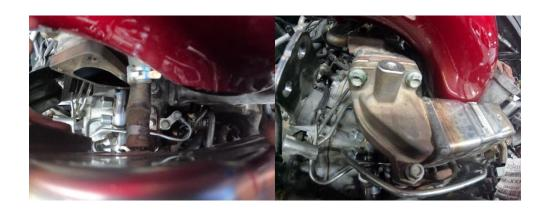
22. Install front EGR mount bolts & torque to 18 LB FT and reconnect front coolant hose.
