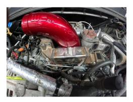
21. Install coolant hose into back side of EGR cooler, then install new EGR gasket from front section to rear section & tighten bolts to **18 LB FT**.
