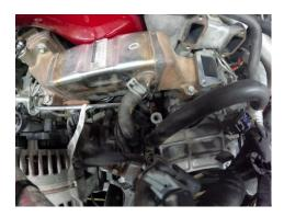
23. Install EGR valve & torque to **18 LB FT**. Verify new gaskets with old gaskets before installing them if unsure of locations to place them.
