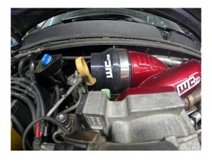
33. Transfer MAF and humidity sensor (if equipped with one) into WCFab Intake Pipe and make sure sensor is closest to the intake horn or it may throw codes due to air flow in wrong direction. If you don't have a humidity sensor, use supplied block off plate.
