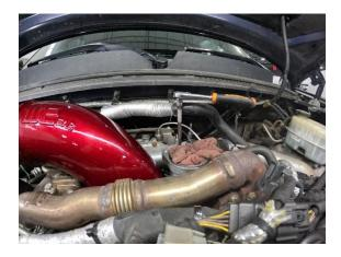
27. Install crossover pipe & reattach wiring to grid heater, MAP sensor, & intake air valve.
