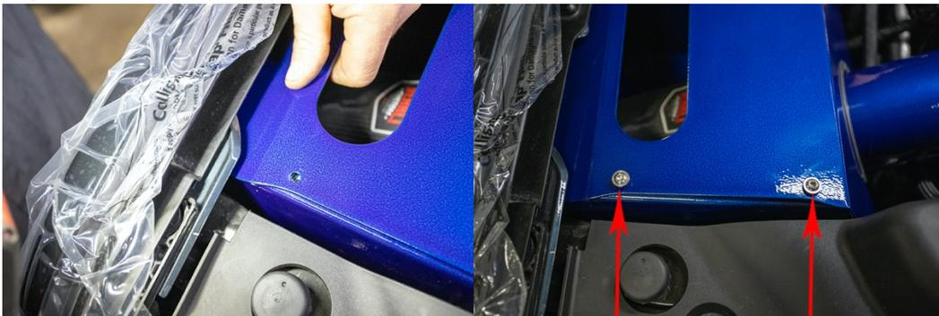
27. Adjust lid to align front air box mounting holes and loosely install supplied fasteners to locate the assembly.
