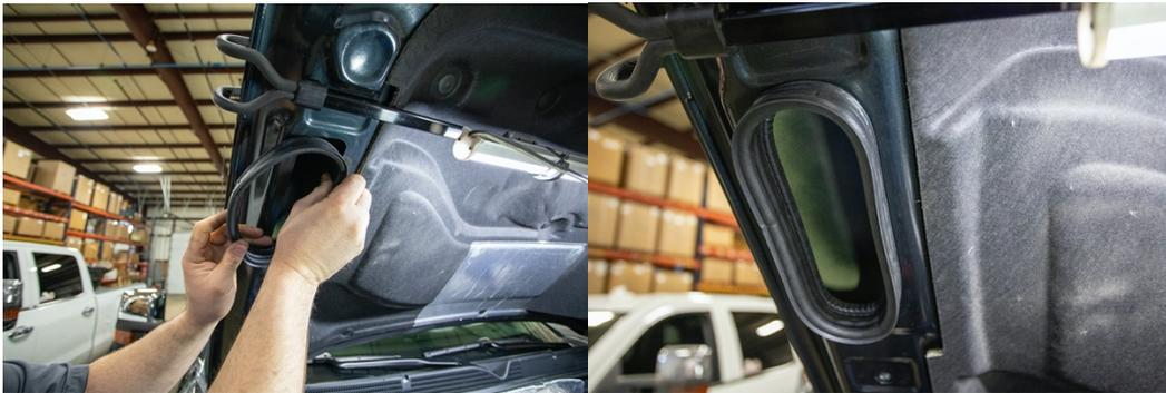
30. Install hood seal onto bottom of ram air hood duct opening as shown.
