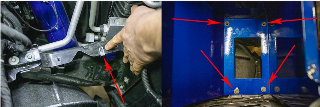
12. Install supplied nutsert, reinstall lower air box and install saved OEM 10mm fasteners from Step 8 working clockwise from rearmost engine side first, completing fender side last. Adjust box alignment as necessary while completing this process.
