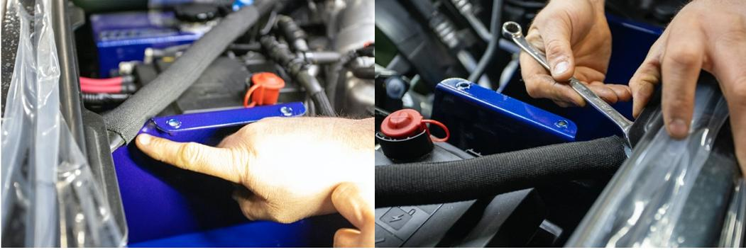
13. Note: Build tolerances vary from truck to truck. Many trucks will require no adjustments for your air box installation. However, on some trucks, the fender brace may contact the air box as shown in this image. To correct this, first loosen the brace at the fender using a 13mm wrench.
