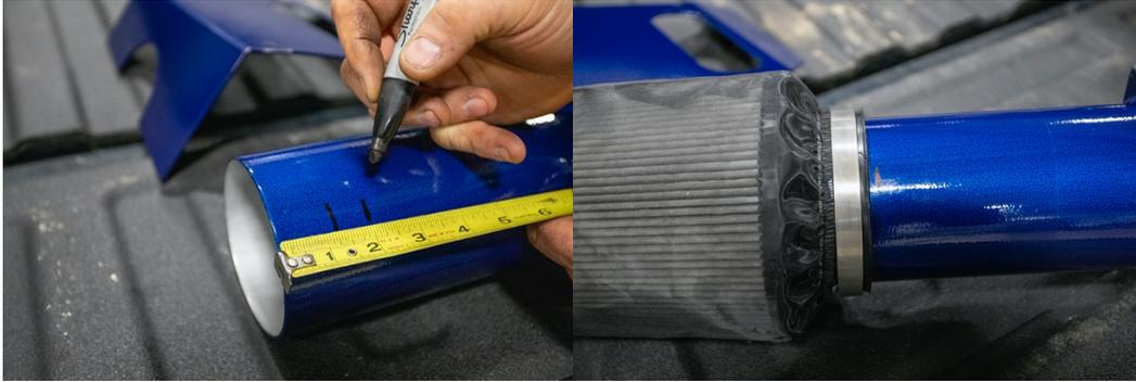
17. Using a tape measure and a marker, place small mark at 2" from filter end of your new intake pipe to help set mounting depth. Install filter onto pipe leaving mark exposed. **Improper filter depth can cause air restriction on your new intake.** Do not tighten filter clamp at this time.
