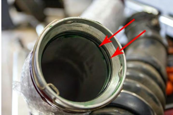
18. Install 2 o-rings, dry, in lower grooves as shown. Once o-rings are fully seated, apply transmission assembly lube (such as Trans-Jel or Dr. Tranny's Assembly Goo) to inside of pipe connection, o-rings, and intercooler outlet to help prevent damage during install. **Avoid using petroleum or other synthetic lubricants which may damage o-ring seals.**
