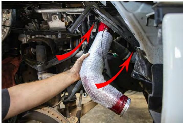
21. Install new intercooler pipe upwards carefully through passenger side wheel opening paying attention not to damage charge air temp sensor.
