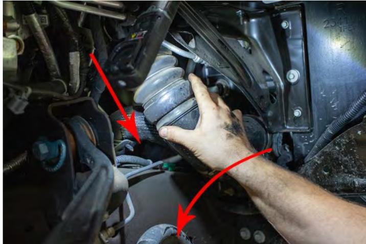
14. Remove pipe by passing it out carefully through passenger wheel well.
