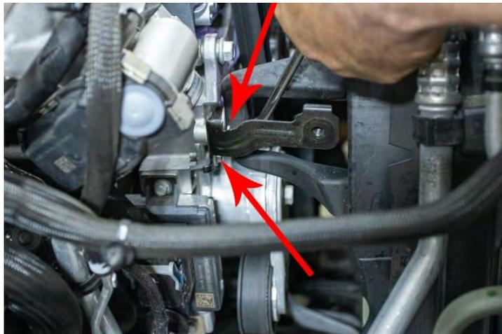
19. Remove OEM Intercooler support bracket from engine as it is no longer required.
