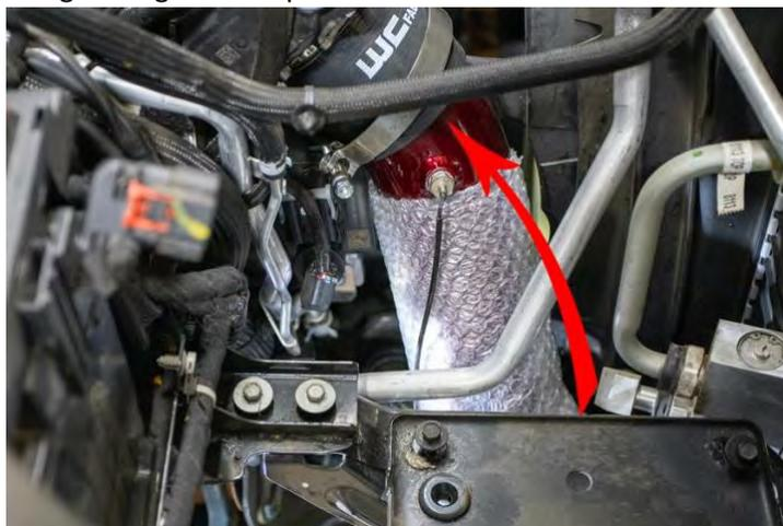
22. Slide pipe into upper boot and slowly put lower end on the intercooler. Make sure to stay square with the intercooler as much as possible.
