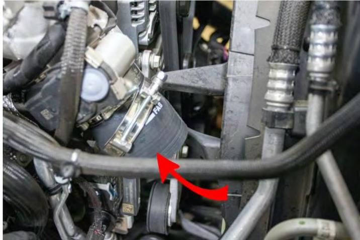
20. Install top boot and clamps onto the engine intake side and leave loose.
