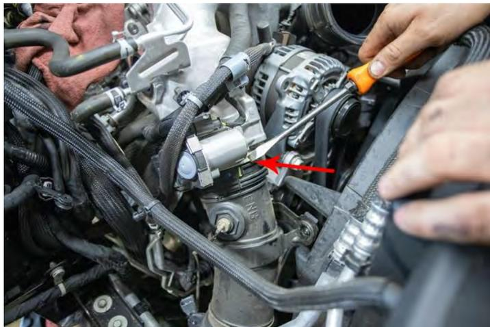
13. Turn lock ring clockwise to remove top connection to engine and slide pipe off of intake flange.
