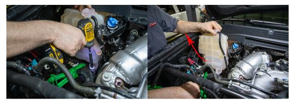
7. Install the new level sensor into your new tank. These are pipe threads and require sealant. We recommend using a liquid pipe thread sealant. Tighten the sensor up and make sure to have the arrows on the sensor facing up. You will also install the overflow nipple just under the cap. **NOTE: White hex sensor needs arrow pointing up, black round sensor needs arrow pointing down**.
