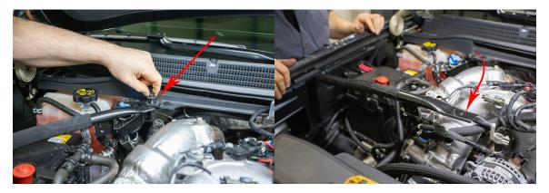
3. Remove the battery hold down bolt and disconnect both terminals. There will be four connections needing to be removed from the junction box on top of the battery to allow it to swing out of the way. Two will be a larger gauge wire with 13mm nuts. The second two will have a quick release tab on them and can be removed with a small flat blade screwdriver. Now, move the junction box out of the way.
