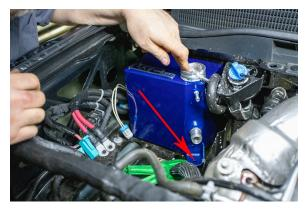
9. Reconnect the factory hoses onto tank. At this time, you can install the overflow hose that came with your new tank. Route so that this in not laying on or near the engine or the exhaust manifold.
