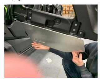
10. Use the new lower door as a template to drill 3 vertical holes.
