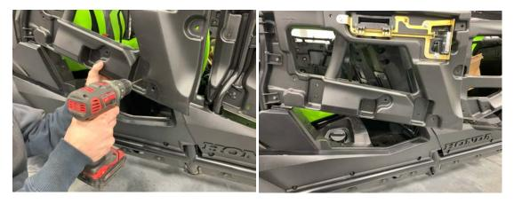
9. From the inside, insert two 1.5" long bolts with washers into the two holes towards the front of the door. Insert two 7/8" bolts with washers into two holes towards the back of the door. Make sure the door is pushed up tight.
