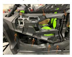
2. Drill four  $\frac{1}{2}$ " horizontal holes into the pre-existing factory markings.
