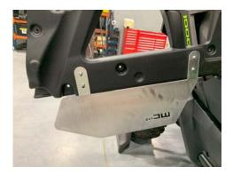
11. Insert 7/8" bolts in the remaining 3 holes. Check all washers, nuts and bolts are in and tighten.
