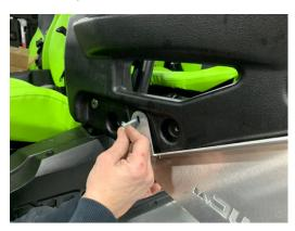
5. Insert 7/8" bolts in remaining 3 holes. Check all washers, nuts and bolts are in and tighten.
