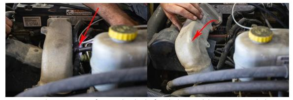
5. Remove wire harness retainer from stud on back of intake horn and then remove intake horn.
