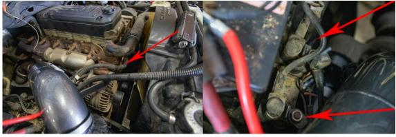
11. If the truck will only see warm weather use, and you prefer a cleaner engine bay appearance, Trace the wire harness pictured above back to the relays near the passenger side battery to disconnect and fully remove the grid heater harness assembly. Take appropriate measures to fully isolate and insulate the empty terminals.
