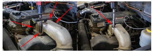
4. Using a 10mm socket and extension, remove intake horn bolts and disconnect dipstick support bracket.
