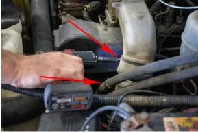
3. Loosen Clamps at the intake horn connection.
