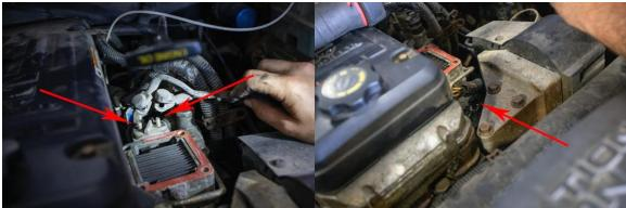
6. Disconnect grid heater "+" connections at rear of grid heater assembly and '-' ground bolt connection from front of assembly.
