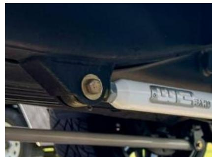
8. Remember, the grease fitting should always point down. Be sure to tighten the jam nut at the front joint against the bar after everything is adjusted and the front and rear bolts are tight.
