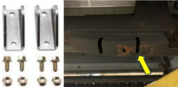
6. You can now install the front traction bar bracket and tighten all bolts. We recommend painting the bracket after the rear mount hole has been drilled out. This will ensure the bracket is protected from the elements and rusting.
