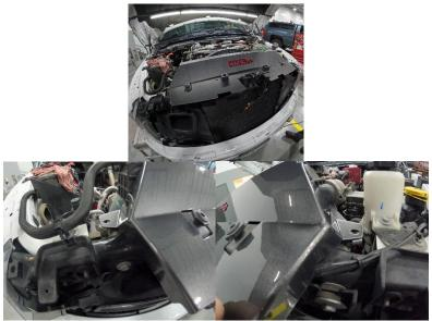
5. The grill can be installed, make sure the bottom two tabs are properly attached before starting any of the other bolts. Once the bottom tabs are attached to the truck start all four of the grille bolts by hand and make sure you have proper clearance.
