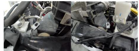
4. Hold the cover in position and start the two outer bolts into the J nuts previously installed. (DO NOT TIGHTEN).
