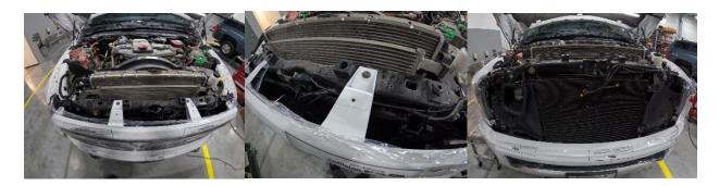
3. Install the two J nuts in the locations shown at the outer tabs on the radiator.
