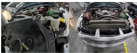
2. Remove the four 10 mm bolts from the grille assembly along the top edge of the grille. Remove the grille from the truck by pulling gently at the bottom edge of the grille out and up at the same time.
