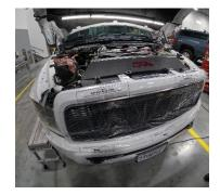
6. Tighten the 6 bolts by hand to the grille and radiator shroud.
