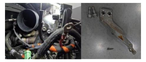
8. Remove two mounting bolts from upper crossover pipe at y-bridge connection and remove it from engine along with intake air valve and heater.
