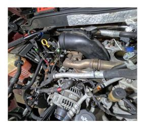
24. Reinstall AC compressor and serpentine belt.
