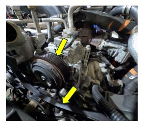
13. Remove upper radiator hose and A/C compressor to access EGR cooler hardware.
