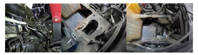
6. Disconnect temp sensor on top of passenger intercooler pipe and release retainer securing pipe to throttle valve and remove pipe from engine bay.
