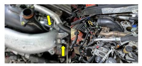
9. Remove PCV port from intake horn and then remove horn from engine after loosening clamp at turbo inlet.
