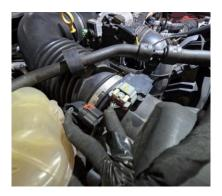
3. Remove intake tube along with airbox/lid.
