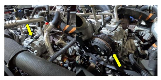
25. Install o-ring in crossover pipe flange then fasten throttle valve/heater (with new gasket in place) and MAP sensor on new crossover pipe and fasten it to Y-Bridge inlet flange. Engine side bolts are torqued to 18ft-lbs and intake air valve bolts are torqued to 89in-lbs.
