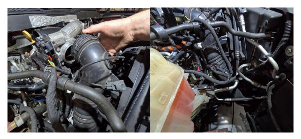
27. Reinstall upper coolant hose to thermostat housing and radiator.
