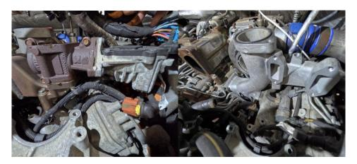
15. Remove Y-Bridge from engine valley. Turbo bolts at pedestal will need to be loosened to allow turbo to be rocked back towards firewall with a pry bar to give access to y-bridge bolts.
