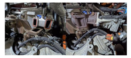
21. Reinstall intake horn and clamp while EGR cooler is still loose and maneuverable.
