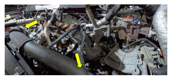
14. Remove front section of EGR cooler.
