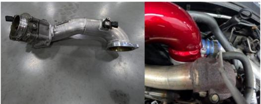
26. Reinstall passenger intercooler pipe between intercooler and throttle valve until you hear an audible "click".
