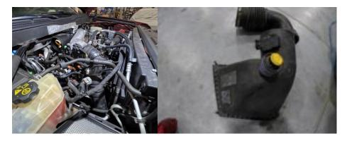
4. Remove electrical connector and power cable at intake air heater, then disconnect connector at intake air valve.
