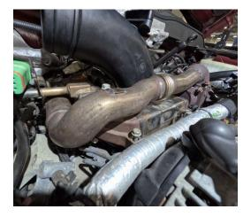
23. Begin tightening down all EGR bolts to 18ft-lbs, starting at passenger side and working towards driver side.
