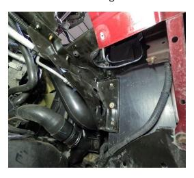
29. Reinstall airbox and intake tube.
