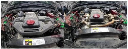
2. Place your new engine cover into position and start all four of the newly provided bolts into the engine. Once they are all started, tighten them equally down by hand to avoid any damage. Install engine oil dipstick.
