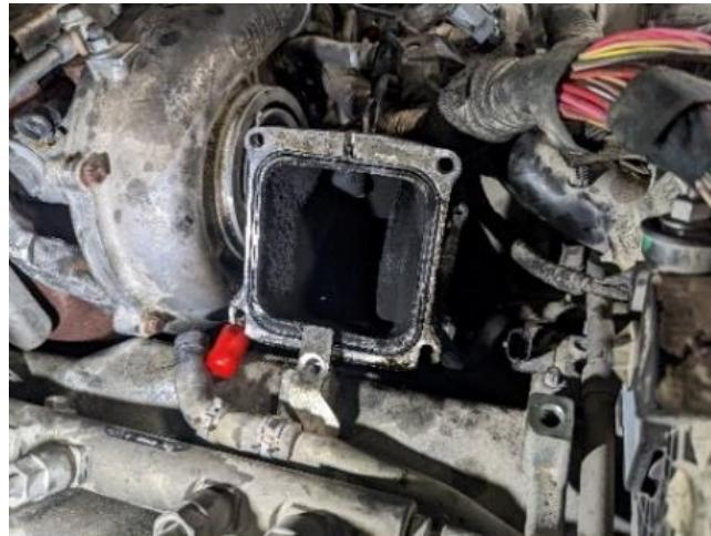
10. Clean up surfaces on intake runners, grid heater, throttle valve and EGR connections.
