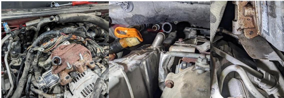
8. Remove front section of factory y-bridge and disconnect fuel pressure regulator connector. Remove fuel line brackets and E8 stud on passenger side intake runner.
