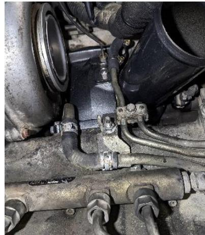
17. Install EGR valve and cooler, up pipe fasteners and coolant hoses.
