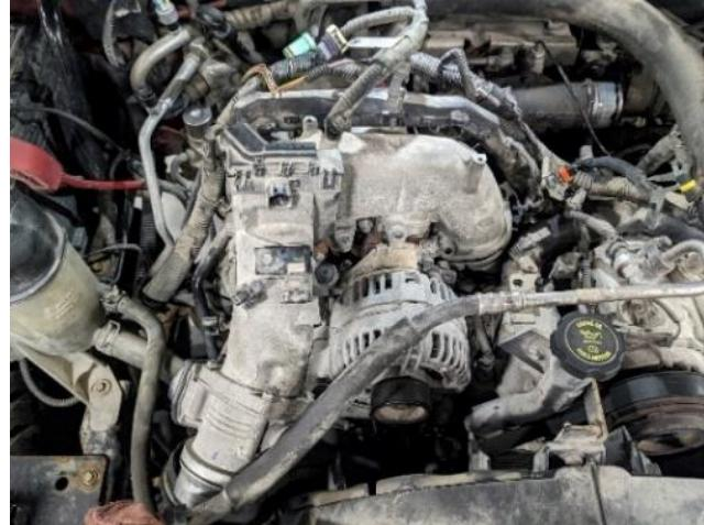
7. Remove EGR valve electrical connector, heater core hose to EGR, rear hose to EGR and 12mm fasteners at up pipe connection to EGR cooler assembly. Remove four 14mm bolts holding EGR cooler to engine. Lightly push EGR back while lifting front near EGR valve to get it over passenger side fuel rail heat shield. Lastly, remove plastic wire guide originally attached to crossover pipe (this will not be reused).
