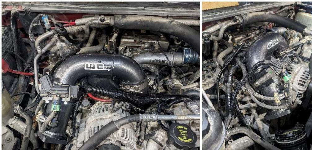
21. Connect passenger and driver side intercooler pipes. Boost test to check for leaks after install or during service on any of installed parts.
