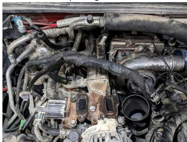
19. Install new crossover pipe with grid heater and throttle valve using supplied O-rings (original gasket will not be used in locations with new O-rings). If extra length is needed for grid heater wiring pull back loom and separate that section. Re-loom or tape electrical harness as needed.
