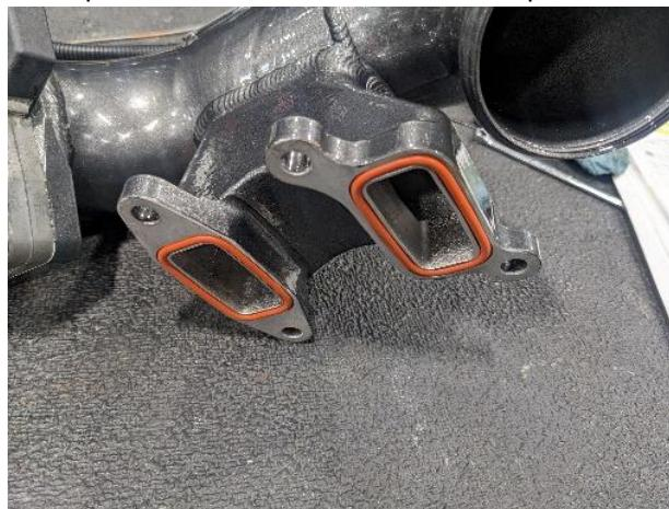
20. Install crossover assembly using factory hardware and torque to 18 FT LB.
