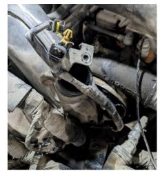
6. Remove crossover pipe as a full assembly and disconnect alternator wiring. Position behind crossover pipe before removal. There are two 12mm fasteners on front bracket and six 12mm fasteners holding crossover pipe.
