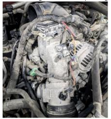
4. Remove intake resonator, driver side intercooler pipe and PCV hose.
