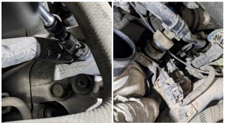
5. Remove turbo intake horn. Disconnect turbo solenoid wire harness & y-bridge temp sensor. Position out of the way.
