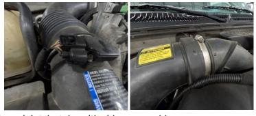
2. Remove factory air intake tube with airbox assembly.
