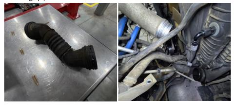
7. Install supplied O-rings in both ends of the new Wehrli pipes dry, then lubricate well once in place. We recommend Dr Tranny's Assemblee Goo.
