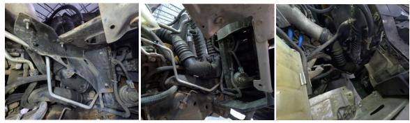
5. Release the retaining clips on the charge pipe with a flat blade screwdriver.
