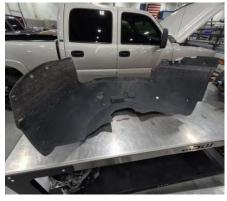
4. Remove air box support bracket and the lower airbox tray.
