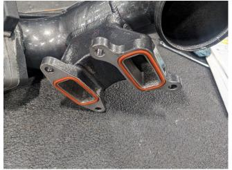
20. Install crossover assembly using factory hardware and torque to 18 FT LB.
