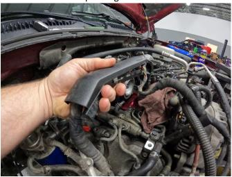
19. Install new crossover pipe with grid heater and throttle valve using supplied O-rings (original gasket will not be used in locations with new O-rings). If extra length is needed for grid heater wiring pull back loom and separate that section. Re-loom or tape electrical harness as needed.
