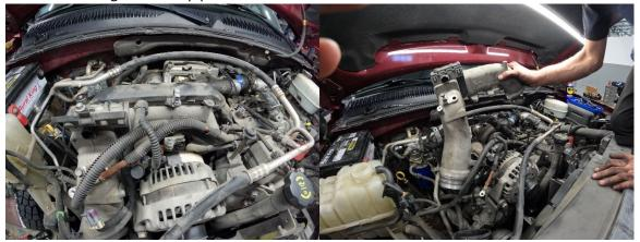
7. Remove EGR valve electrical connector, heater core hose to EGR, rear hose to EGR and 12mm fasteners at up pipe connection to EGR cooler assembly. Remove four 14mm bolts holding EGR cooler to engine. Lightly push EGR back while lifting front near EGR valve to get it over passenger side fuel rail heat shield. Lastly, remove plastic wire guide originally attached to crossover pipe (this will not be reused).
