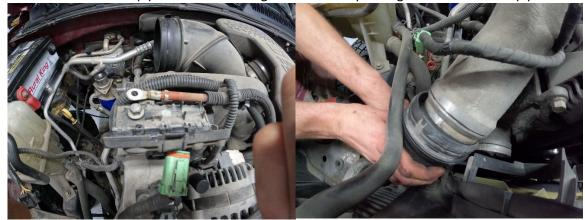
4. Remove intake resonator, driver side intercooler pipe and PCV hose.
