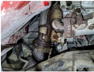
• Remove three 17mm mounting bolts at base of turbocharger.
