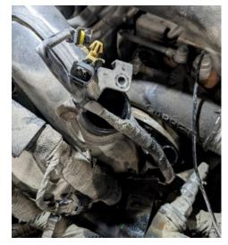
6. Remove crossover pipe as a full assembly and disconnect alternator wiring. Position behind crossover pipe before removal. There are two 12mm fasteners on front bracket and six 12mm fasteners holding crossover pipe.
