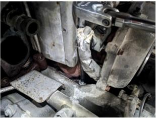
• Use a pry bar to move turbocharger gently to gain access to y-bridge bolts.
