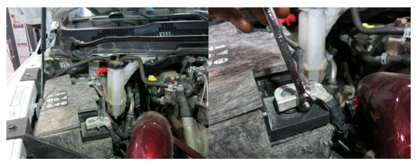
2. Drain coolant. This is at the driver's side of the radiator at the bottom. Unbolt the power steering reservoir and push to the side. You can then reach down to it.
