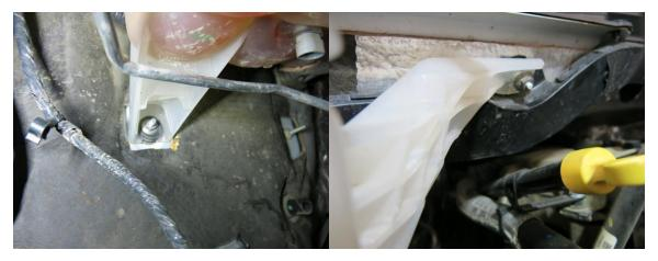
10. Remove the coolant tank.
