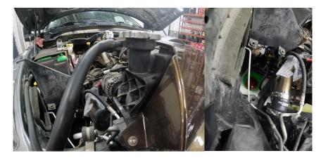
4. Remove the four 10mm nuts holding the tank to the firewall.
