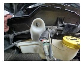
5. Remove the heat shield by removing the two push in retainers as shown below.
