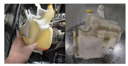
7. Install the provided plug into the filler neck of the new overflow tank.
