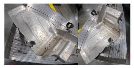
6. The stock tank can now be removed through the wheel well opening.
