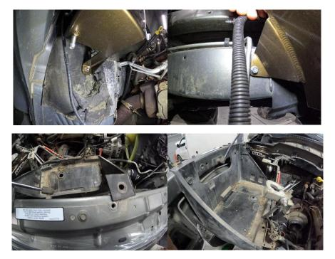
10. The line connecting to the bottom of the coolant tank will need trimmed approximately 6-8 inches on the new tank. A clamp will be installed at the coolant tank to secure the hose.
