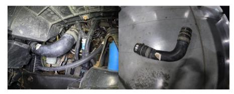
10. Clean the intercooler outlet and install the new boot only tightening the clamp at the intercooler. Install the boot at the intake air valve.
