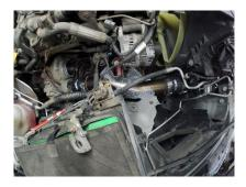
9. Remove the cold side intercooler pipe from the driver side of the engine compartment. This has one clamp at the intercooler outlet and one at the intake air valve.
