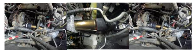
8. Tighten the remaining clamps when proper positioning has been achieved.
