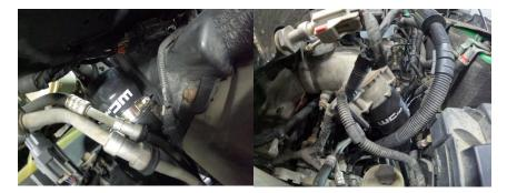
11. Install the new pipe into the boot at the intercooler and rotate intercooler pipe into the boot at the intake air valve. Once properly positioned tighten the remaining clamps.
