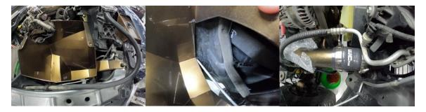
9. Using some Assemblee Goo or similar product, install intake pipe into boot at turbo inlet and position it so tube lays into box and has proper fitment into turbo and box.
